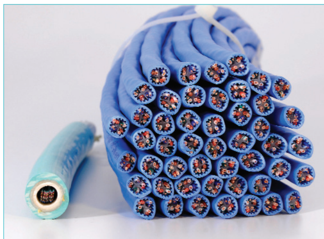
48 “Reduced Diameter” CAT 6A Cables are Required to Serve the Same Number of Ports as One 0.58 in Cable | Photo LAN874
